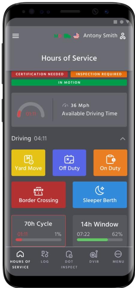
The "Driving" status is recorded automatically 10-15 seconds after a vehicle starts moving. When the driving ends, you should stop, and wait up to 20 seconds until the ELD device recognizes the end of the Driving event and the Status Switch interface becomes active again. Only after that can you turn off the engine.
