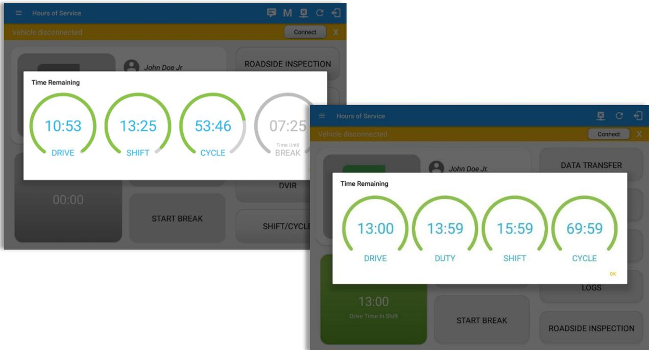
The time remaining clocks are color coded to match the time remaining panel.
