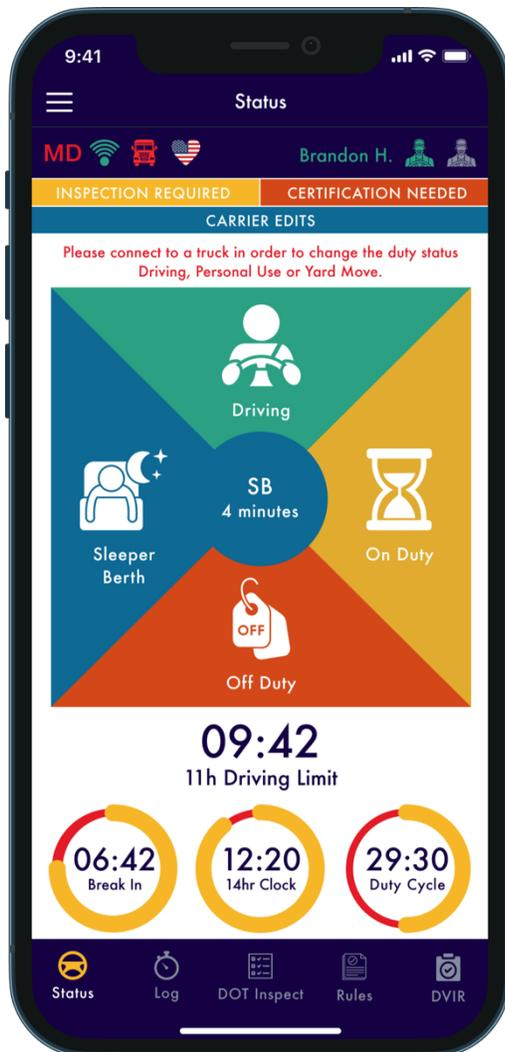
The "Driving" status is automatically recorded within 10-15 seconds after the vehicle begins moving. When driving concludes, it's important to stop and wait for up to 20 seconds until the ELD device acknowledges the end of the Driving event. Only then should you proceed to turn off the engine.
